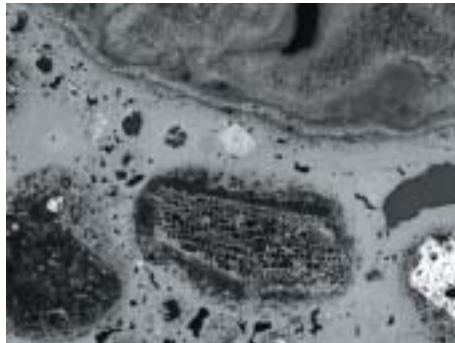
Left Reflected light micrograph of polished section of Yandi fines showing core regions of porous earthy goethite (top and left), fossil wood (centre) and hematite (right) enclosed by porous zones and cemented by dense colloform goethite.
