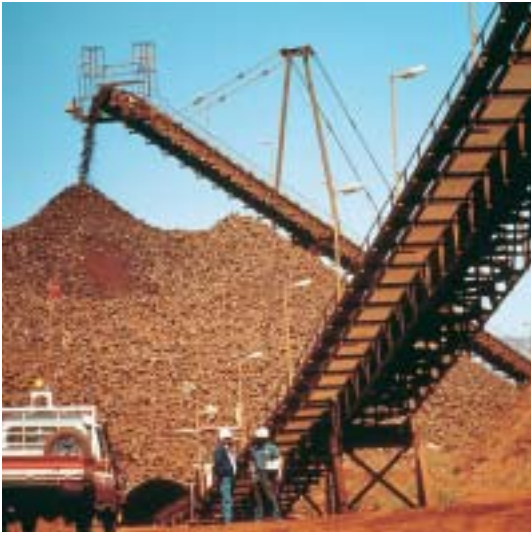
Left Primary crushed ore stockpile at Yandi.
