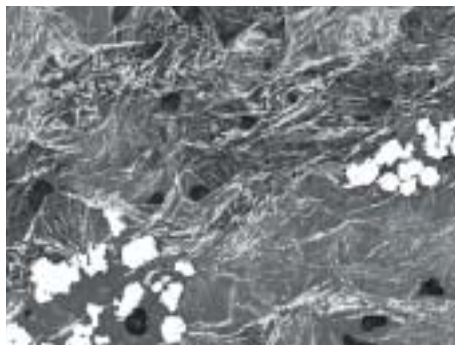
Left Marra Mamba ore (Orebody 29) showing goethite replacing fibrous BIF iron silicate minerals, with areas of martite crystals (white) in quartz. Black areas are pores. Reflected light micrograph of polished section. Field of view is 0.69mm across.
